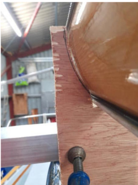
An accurate line was spiled on to scrap ply.
