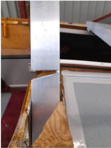
A gusset was cut out of the frame.
