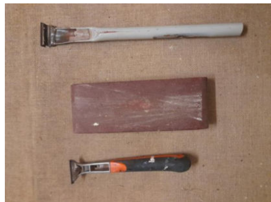
The scraper that worked along with the long handled modified one for inside the keel boxes and the 4-inch sanding belt on a block.
