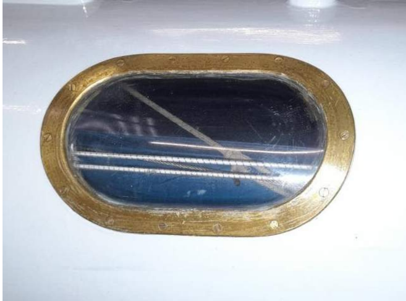
The after port light after having matured for a season's exposure to the weather.
