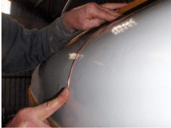
Taking the curve of the hull with copper wire
