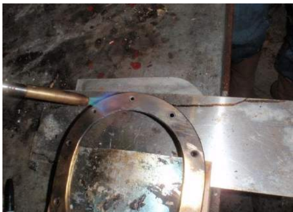
Cherry Red. Note the sheet metal used as heat shield.
