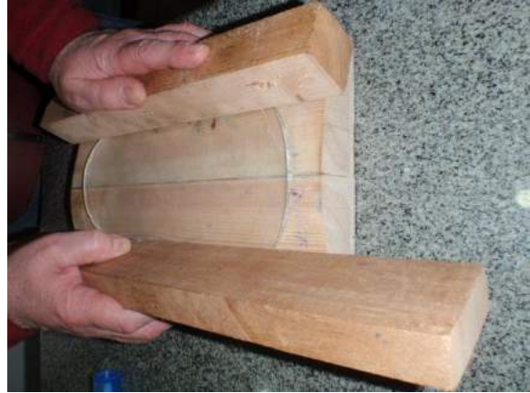
The wooden former being used to re shape the Perspex which bent very easily.
