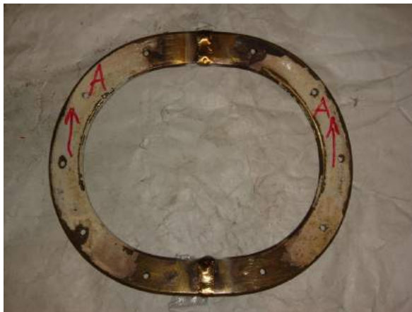
The forward port light roughly welded.
