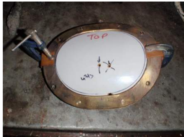
The now cleaned up welds and using the wood cut out as a former.
