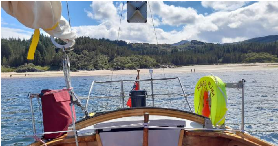
Sugar Plum sporting an octahedral radar reflector.
