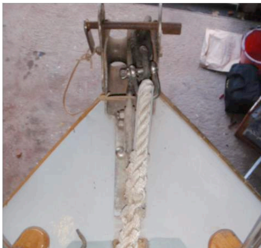
The cheek pieces on the stem head roller with the keeper pin. (How did that stainless steel go rusty?) Note:- to stop any chaffing the bridle is chain as it goes over the rollers, the shackle is wire locked and the bridle is moused onto the bollard.
