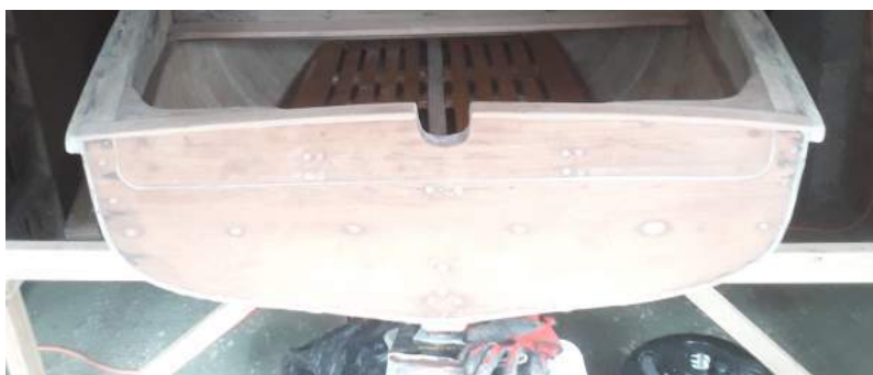
Transom plugged ready for coating
