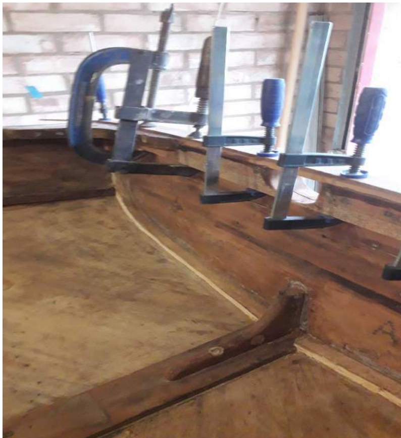
Reinforcing strip of Agba veneer
