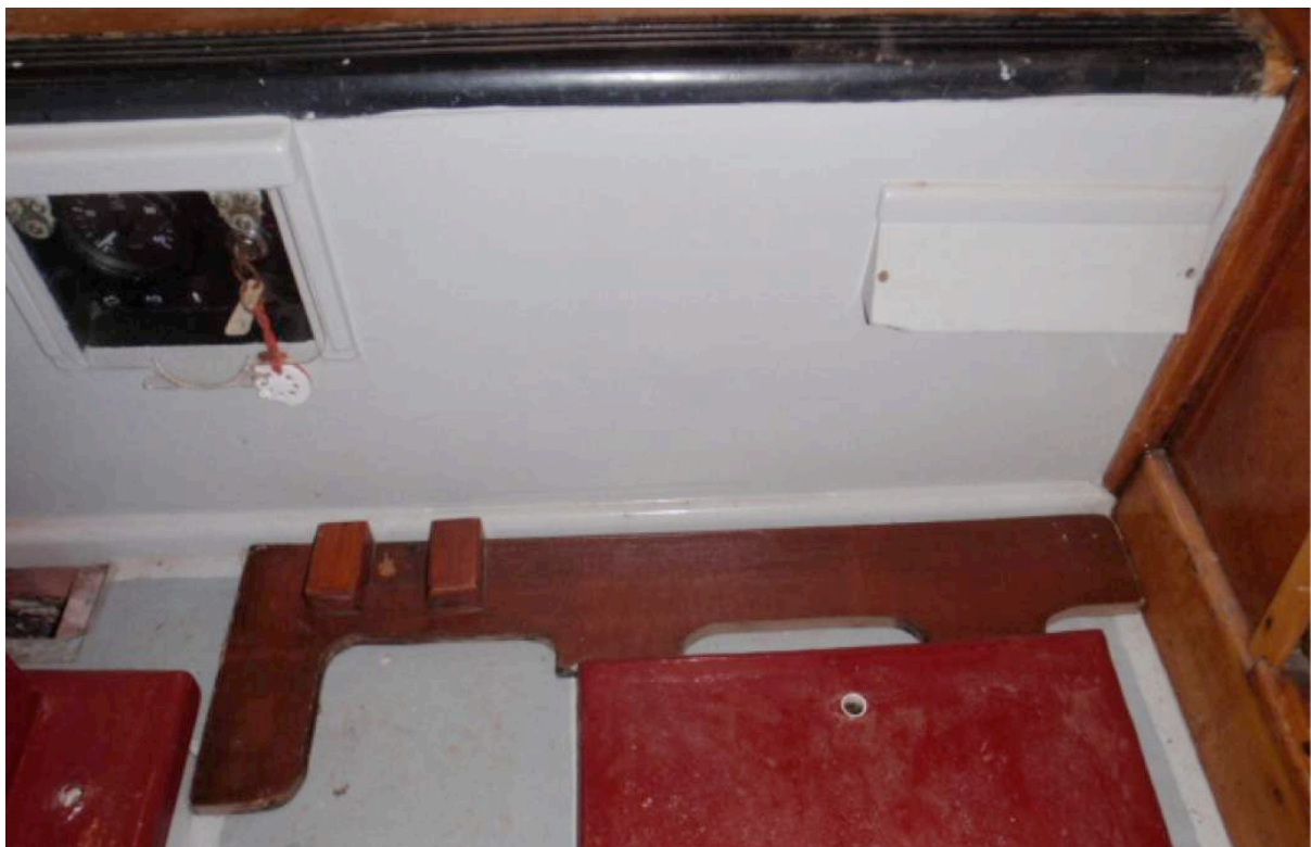
The self locating load spreader boards with lugs to locate the feet of the crutch.
