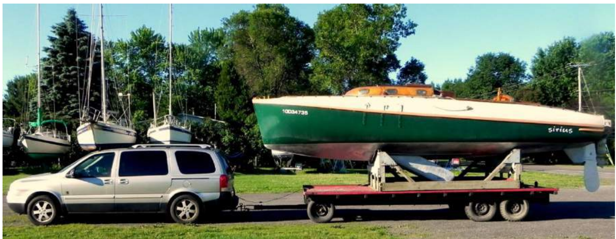
A33 Sirius being towed by Michel Lapierre in Canada on a low-loader. Due to the height of the trailer and frame, the rudder was left fully extended.
