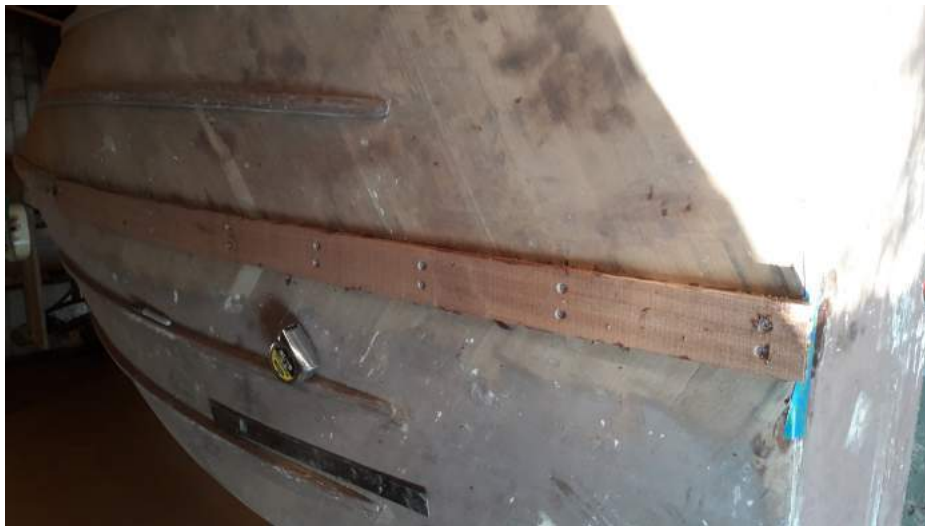
New Sapele strips for the keel
