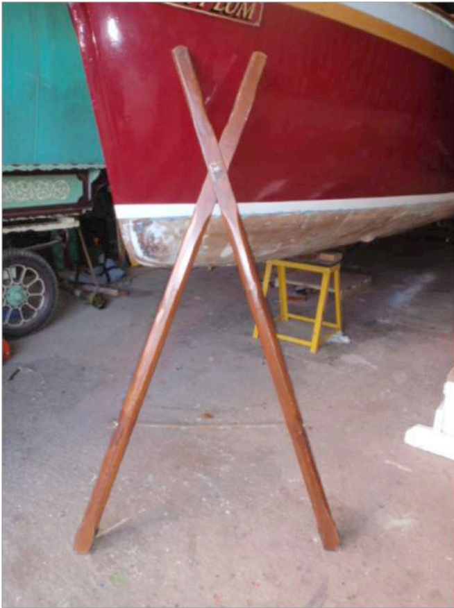
The crutch made to take apart. A scrap of carpet is used as padding.
