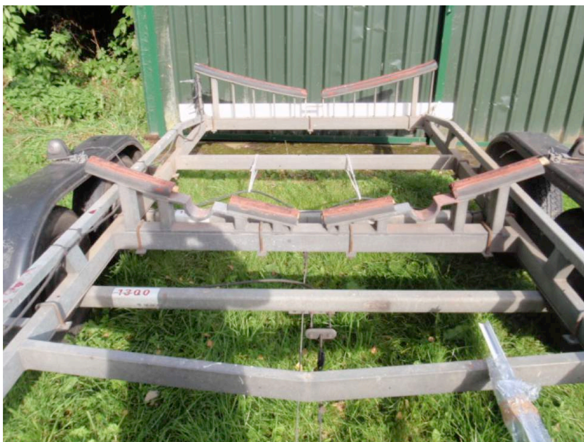
The main cradle of the trailer showing the recesses for the keels to be lowered into once the limit stop blocks have been removed.
