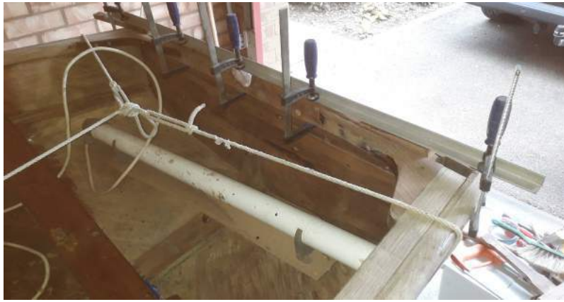
Hull to transom joint clamping arrangement
