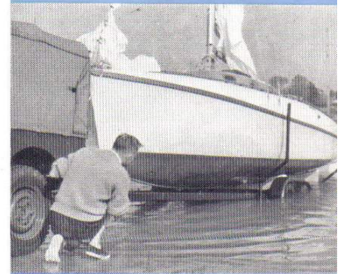
The low-loading trailer is safely submersible for launch and recovery. Special brake-washing arrangements are provided.
