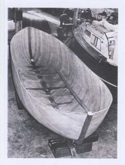
This hull is manufactured by the special Fairey Marine hot-moulding technique of laminated Agba, with seven laminations of  $2\frac{1}{2}$  mm.
