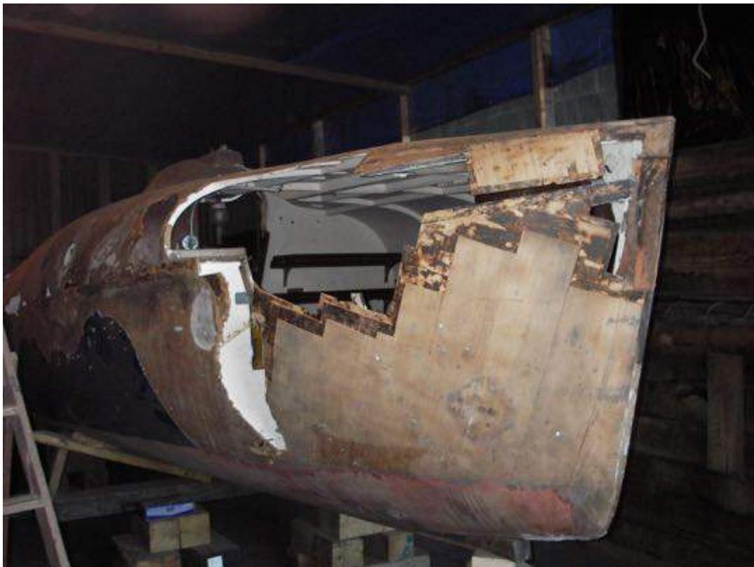
The huge hole in the starboard side
