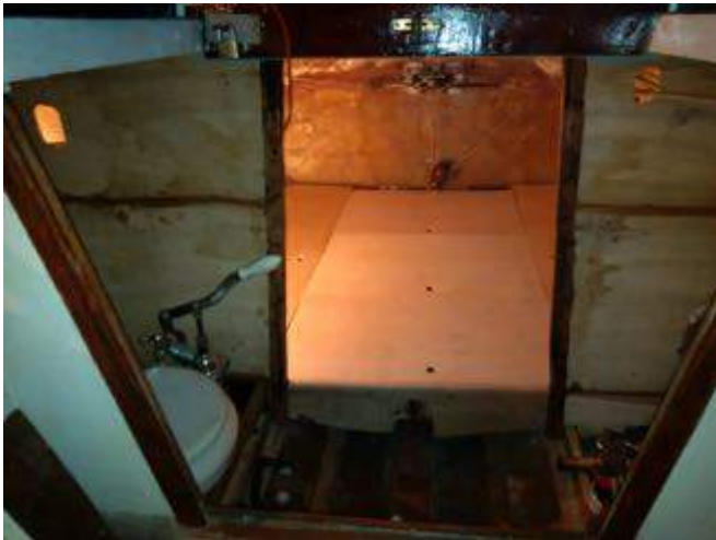
4 Bulkhead details (note rudder control holes)
