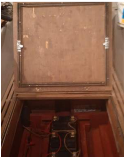
Inside of cockpit hatch showing the locks from below
