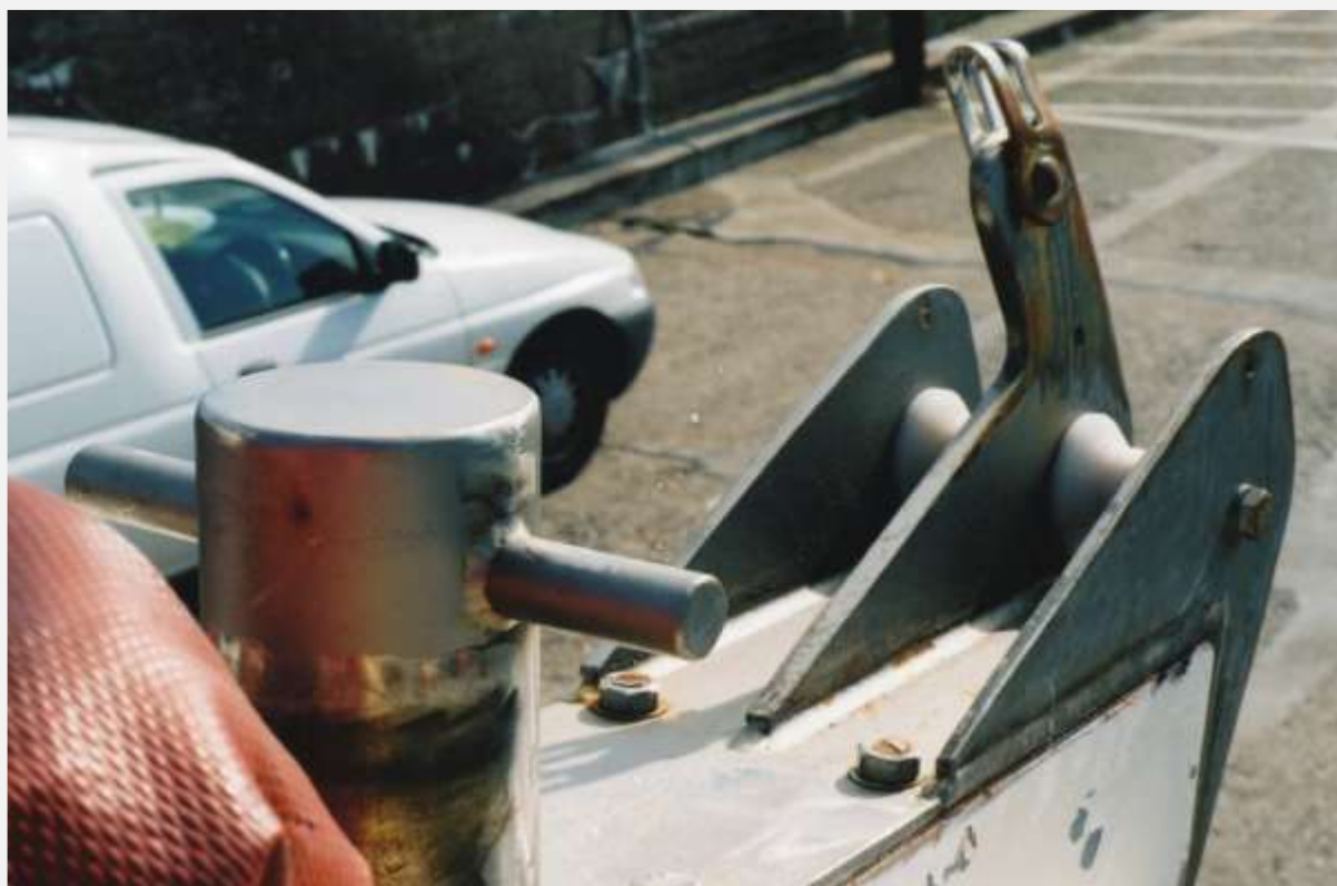
The bow fittings and Sampson post which proved to be so strong
