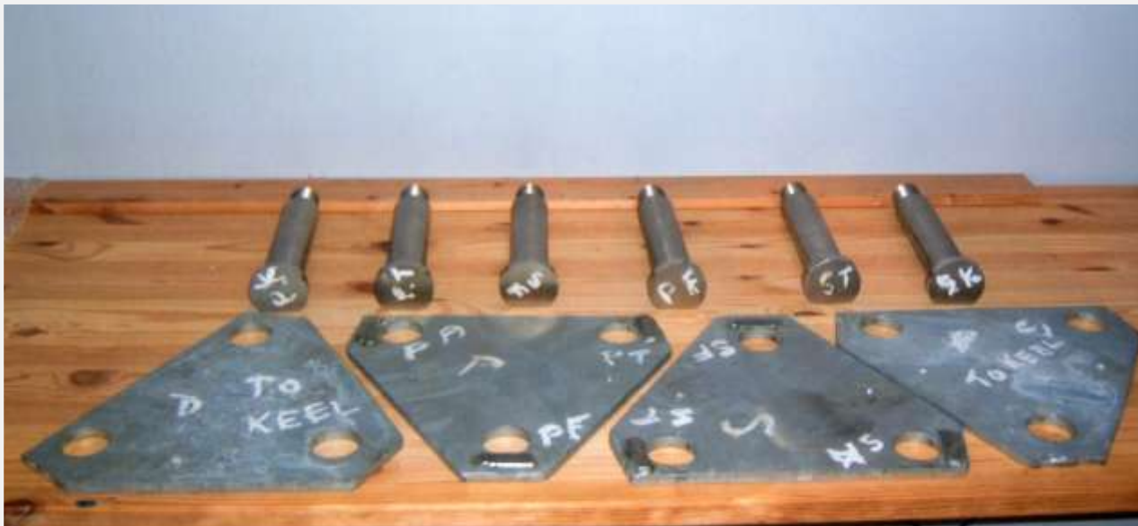
New keel bolts and pressure plates
