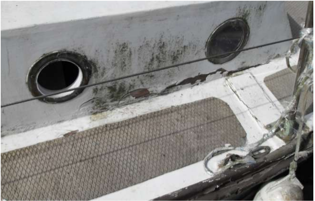
Coachroof side, and deck damage
