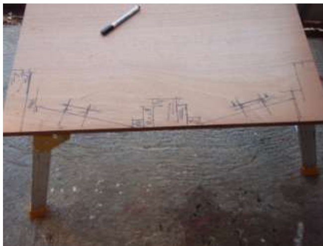
Marking out the forward bulkhead doubler
