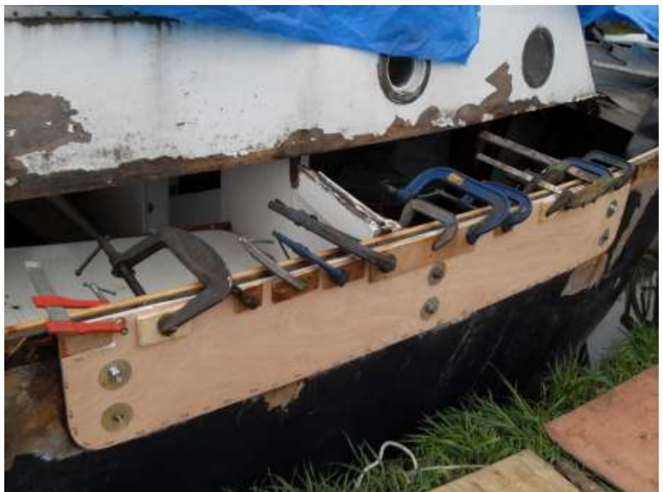
Repairs to the gunwhales where the chainplates are located
