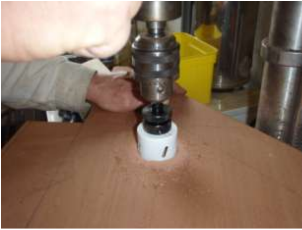
Cutting the tube holes
