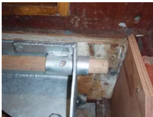
Marking the centres for drilling the tube holes.
