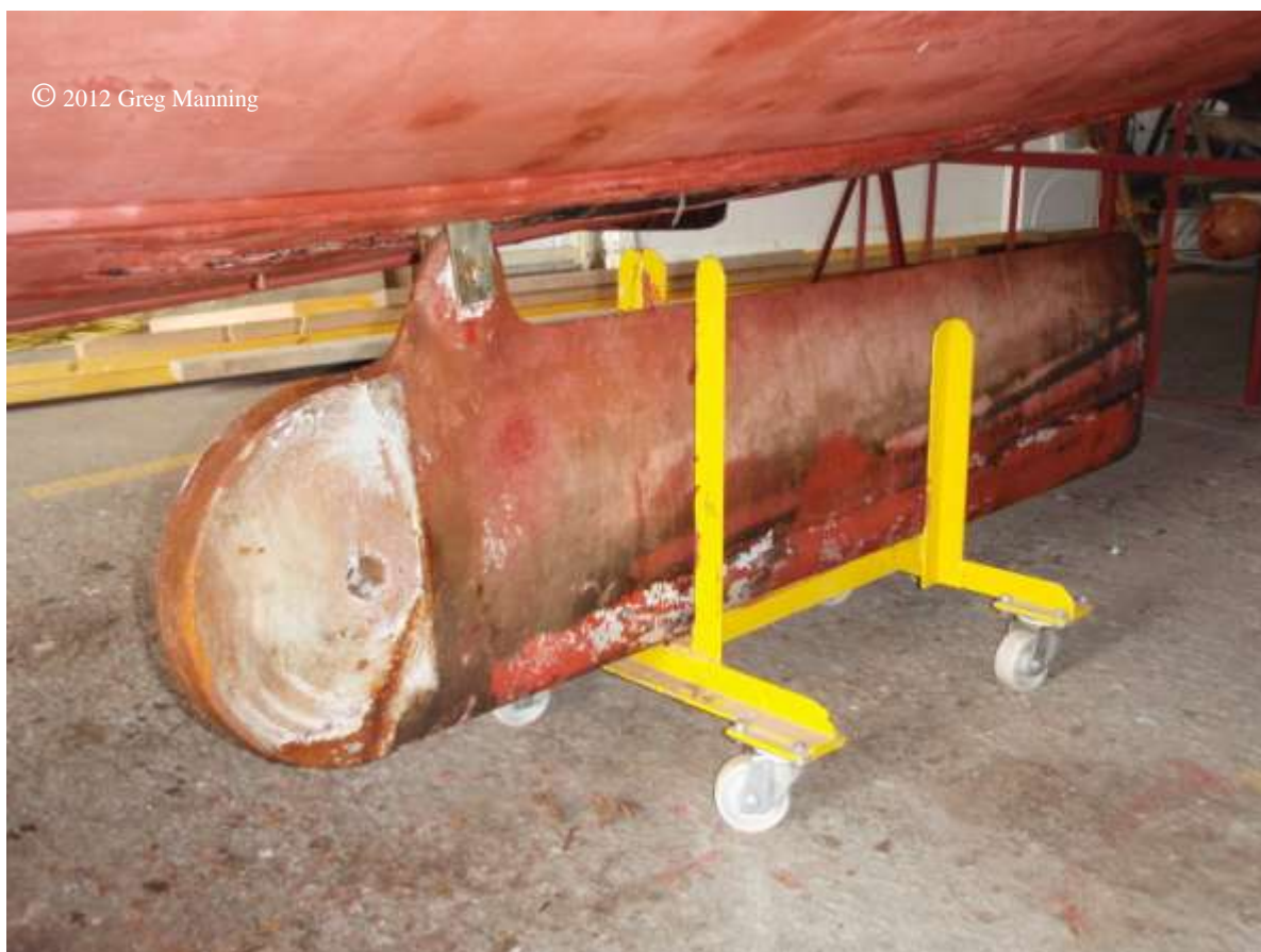
The keel is easy to get in and out this way
