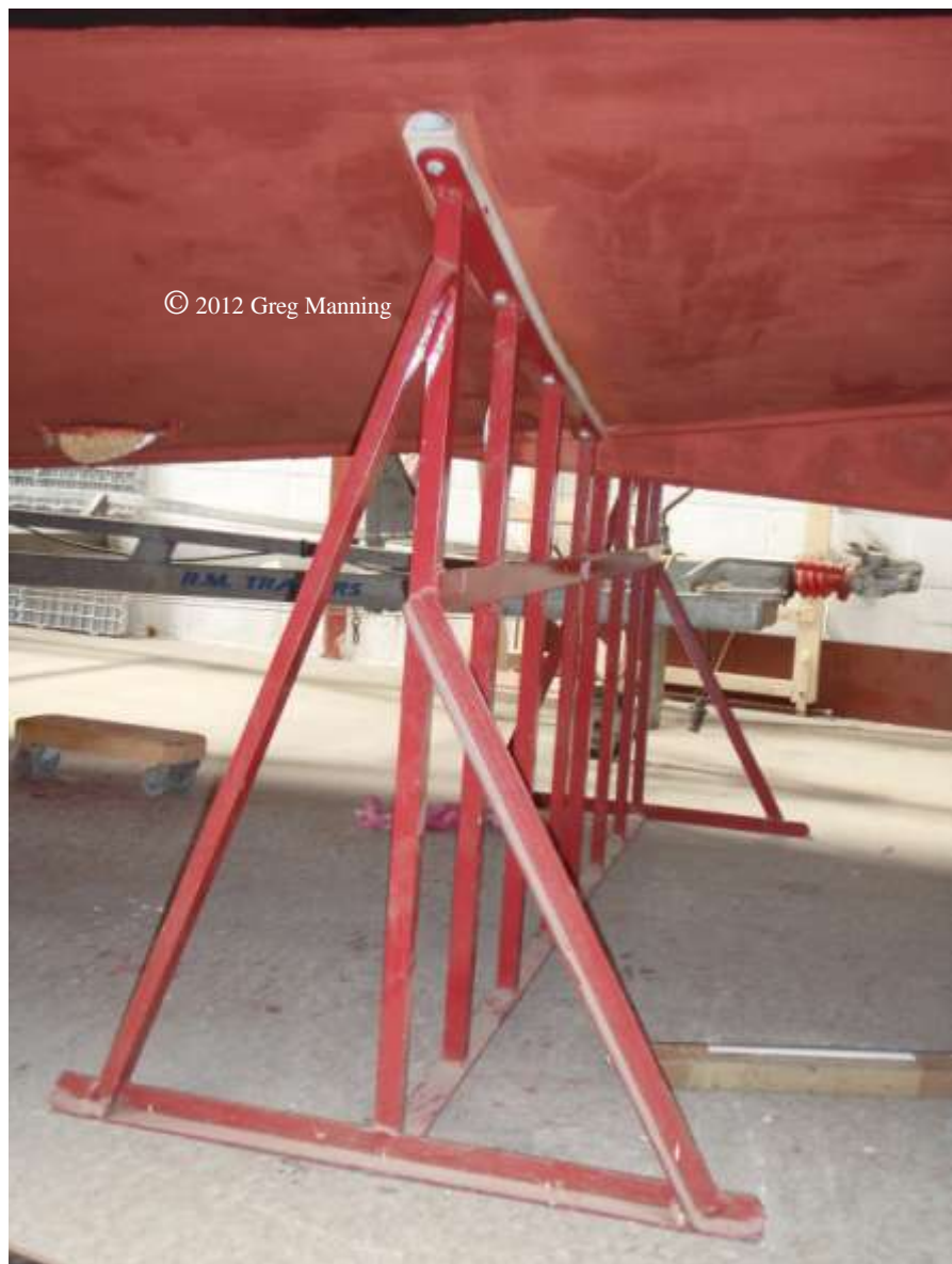
A cradle for the aft bulkhead
