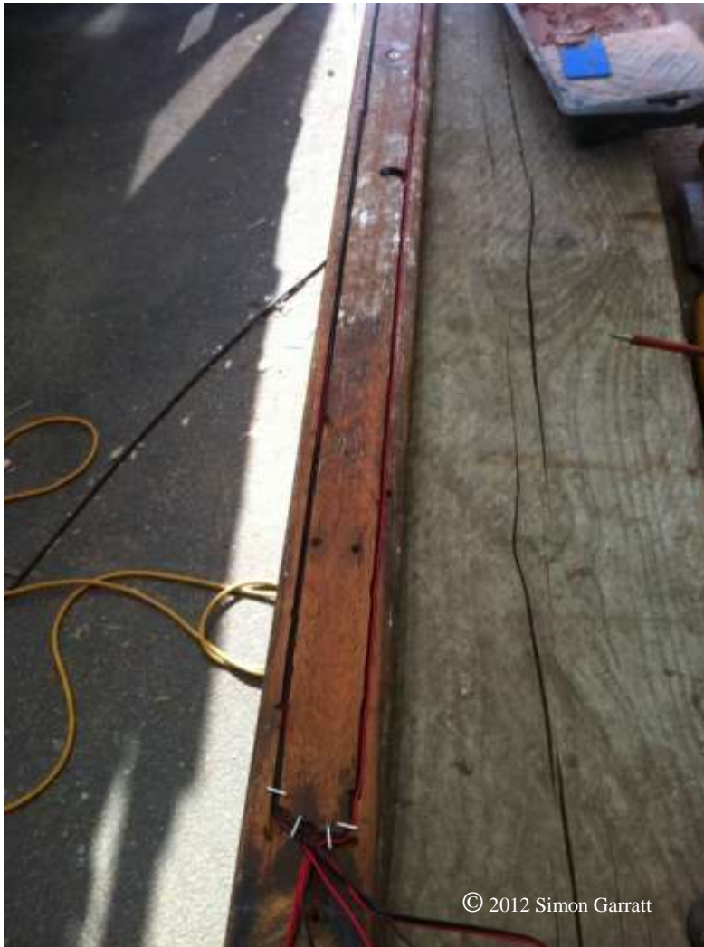
Cable routed in- to the un- derside of the aft toe rail.
