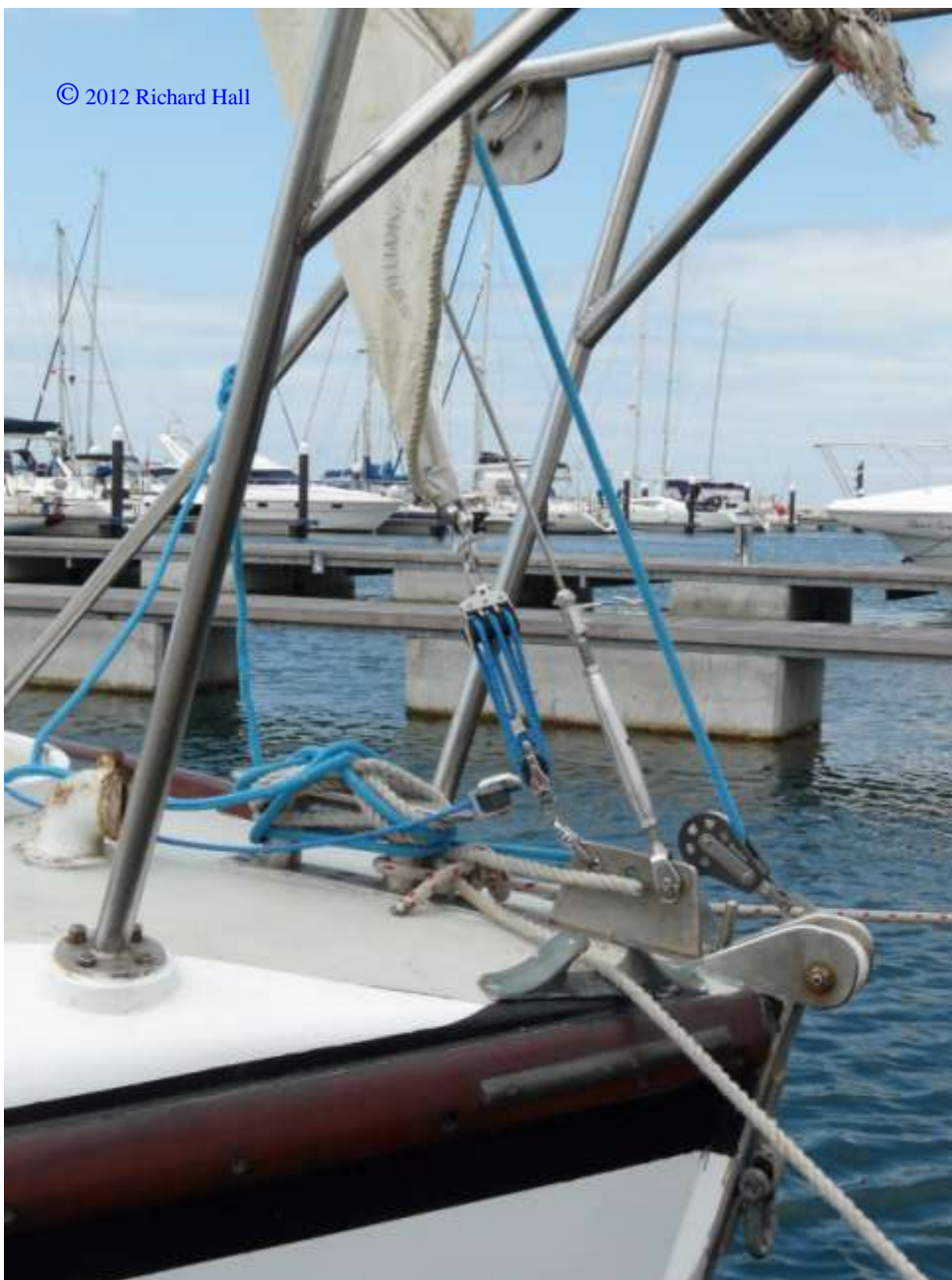
Fig 4: The system for handling jibs from the forehatch
