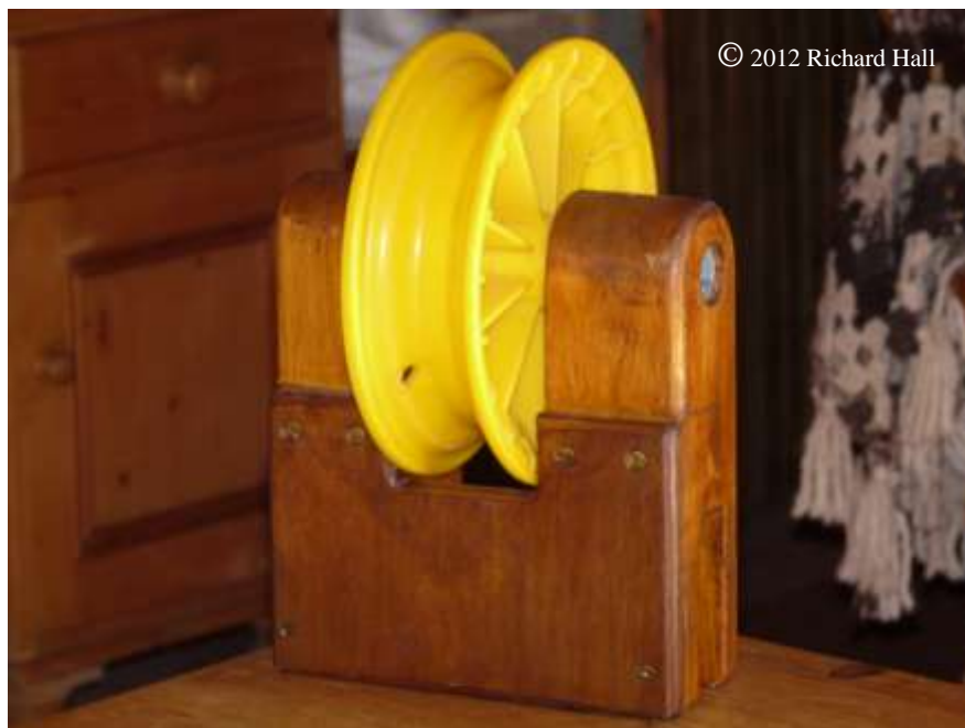
Fig 5: The roller for moving the mast
