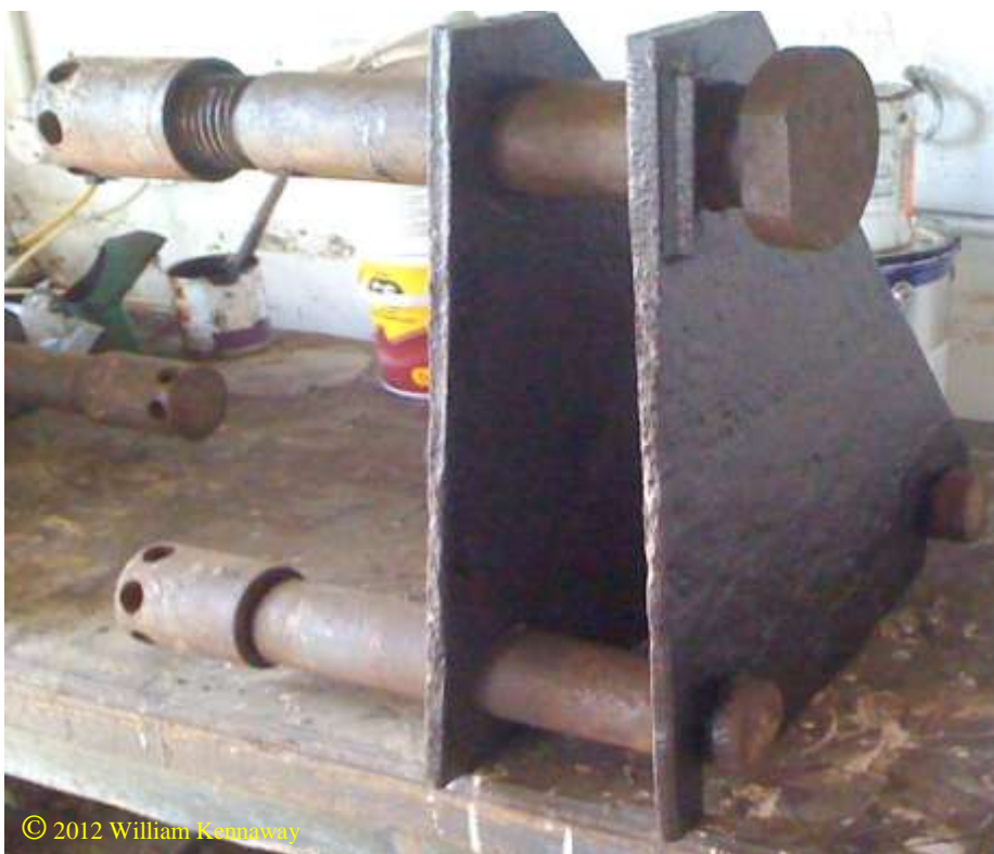
Pressure plates and bolts assembled outside the boat
