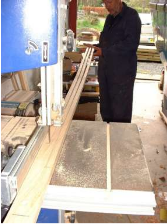
The band saw cutting the slits
