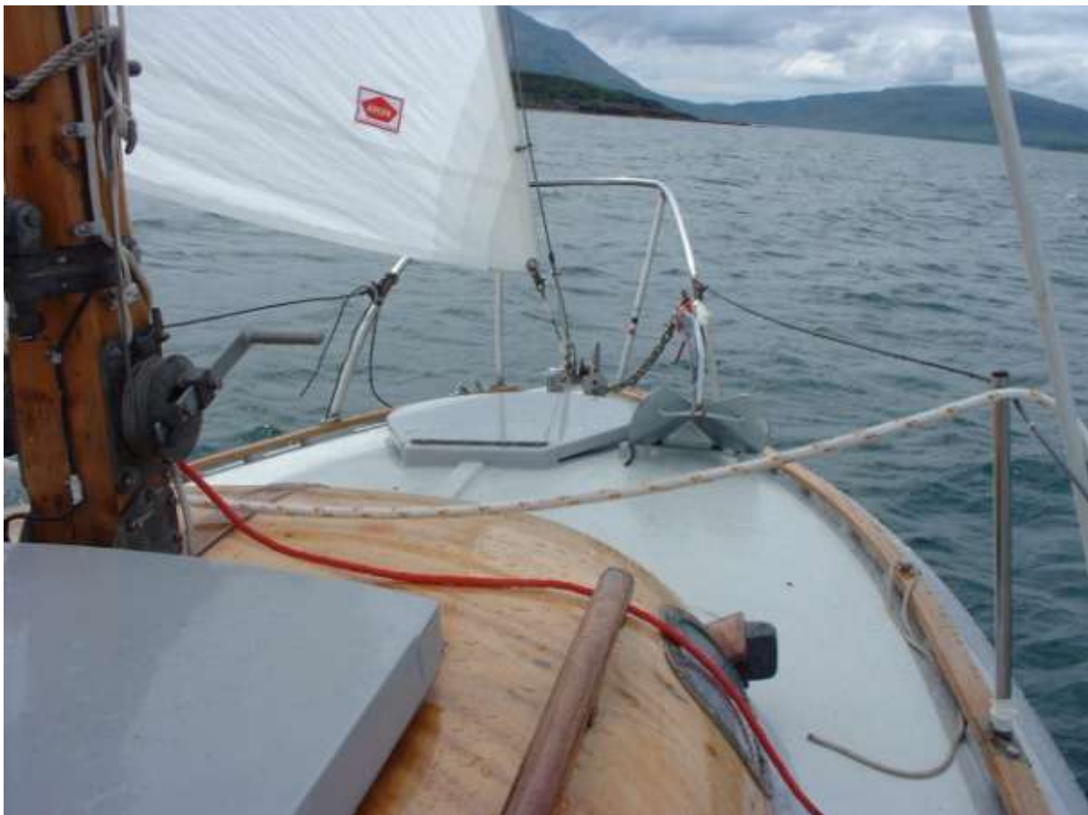
The finished Toe-rails in action
