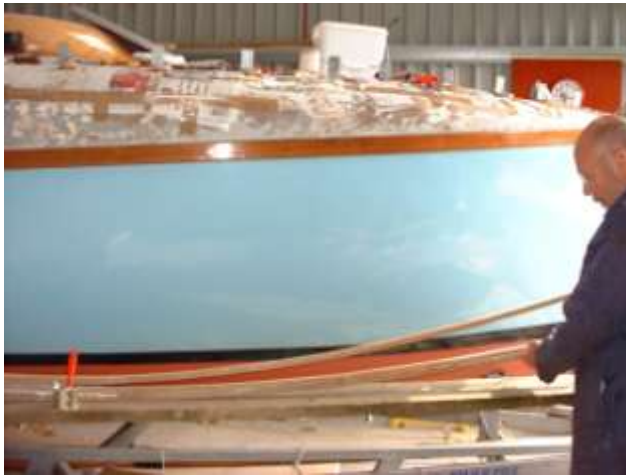
The toe rail slit ready to fit
