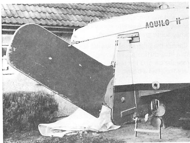
To reduce swinging when moored, the stock is drilled-out for about 6 inches and the rudder supported by two guys.
