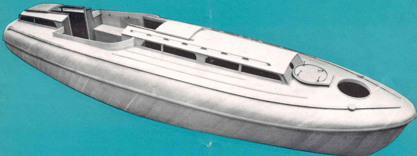
An Atalanta 31 hull part-completed to stage 1 (see below). In this form all the difficult boat-building work has already been done—the hull is assembled complete with deck, cockpit and coach-roof etc.
