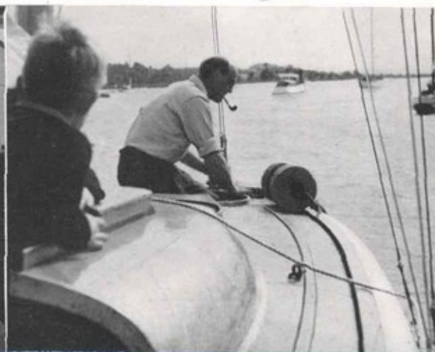
Working Atalanta can be done without going on deck. Setting and handling foresail and mooring can be handled comfortably from the forehatch.
