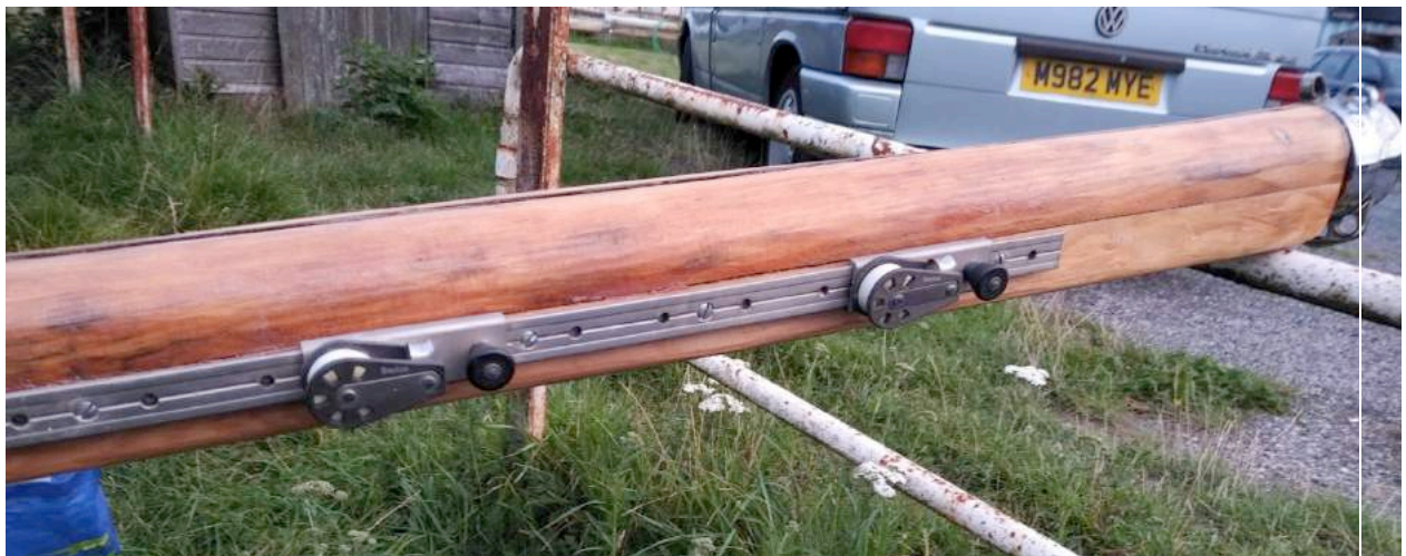
Figure 6 Boom reefing added
