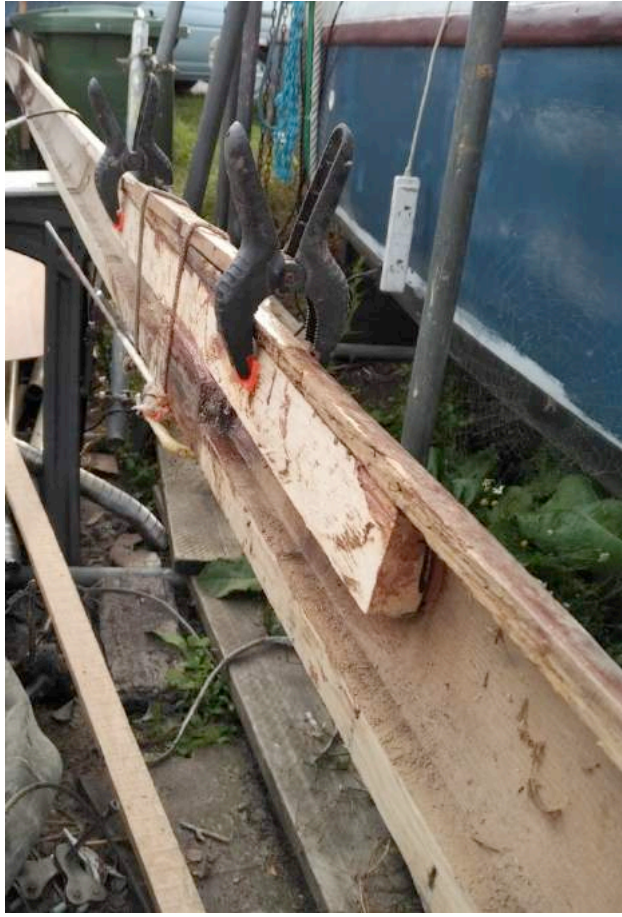
Figure 15. Spruce splines epoxy glued inside crossbeams.
