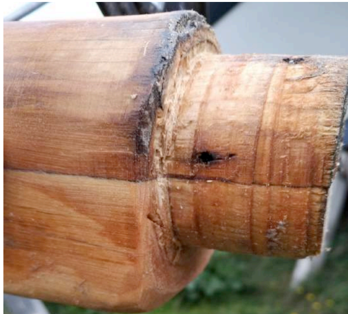
Figure 4 Boom end shaped for new mainsheet end fitting
