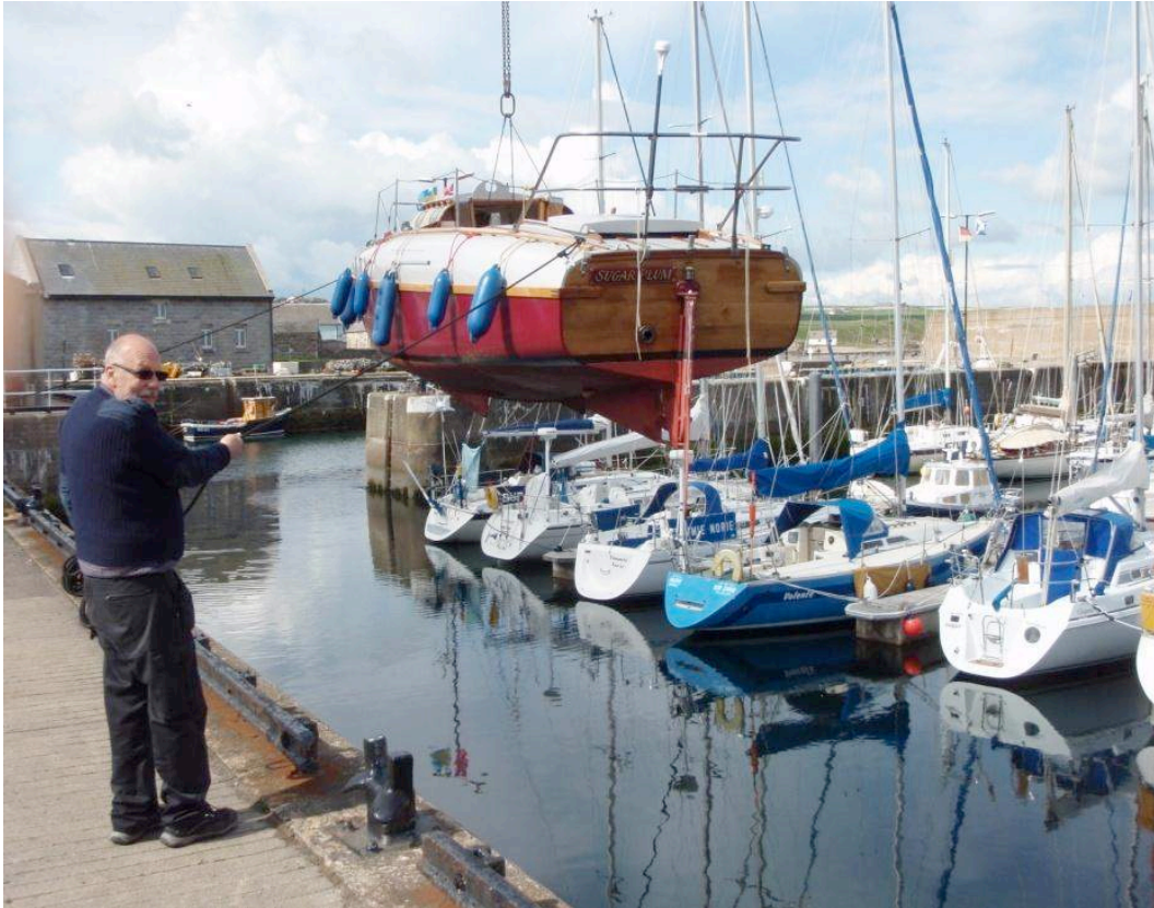
Sugar Plum being launched the way Fairey intended, with an internal sling to correctly take the weight. The picture is at Whitehills a few years ago.
