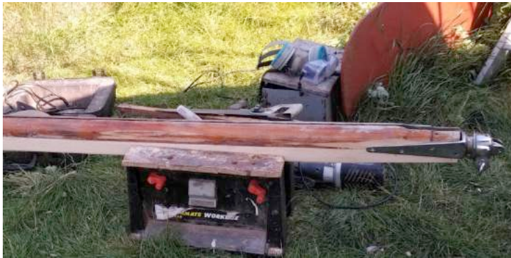
Figure 2. Old top section glued to new lower
