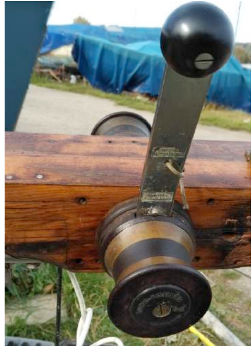
Figure 33. Winch fitting complete.
