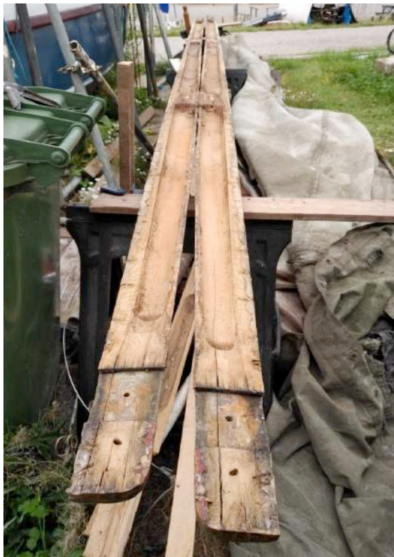
Figure 8. Mast sections separated – clean break along joins.
