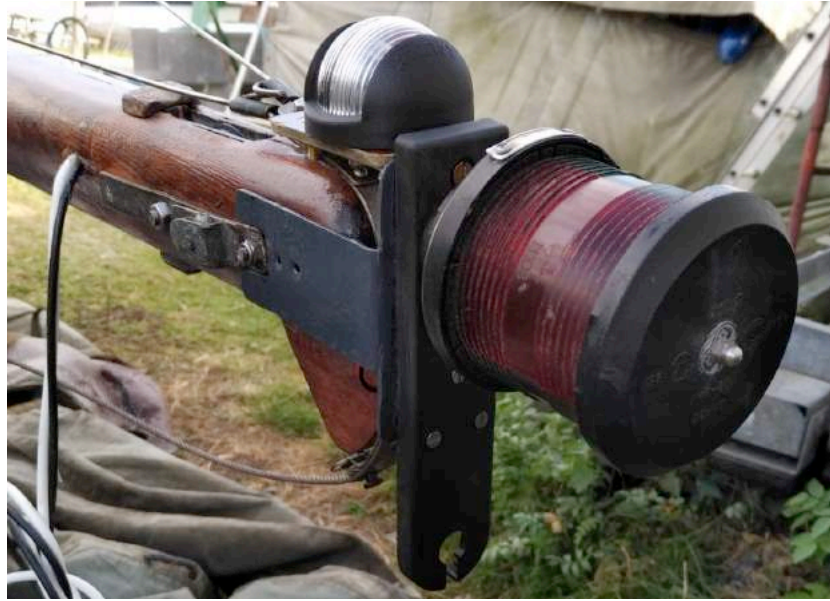
Figure 29 Masthead Nav light & VHF fitting.
