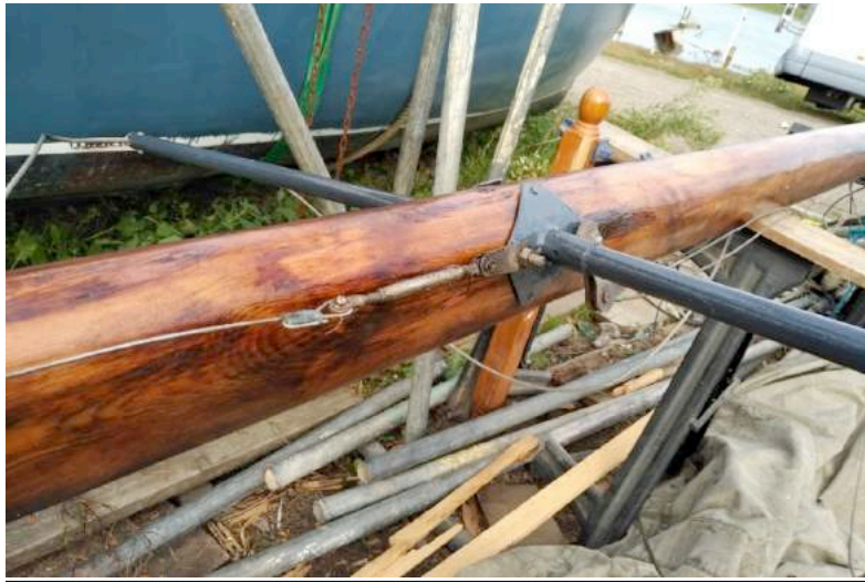
Figure 27. Spreaders, jumper stays & lower shrouds attached.
