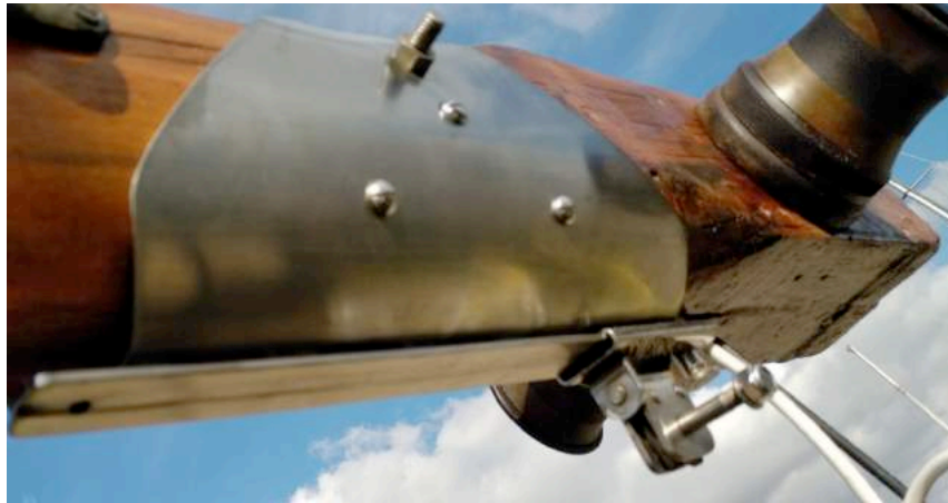
Figure 30. Stainless steel custom sliding gooseneck fitting.
