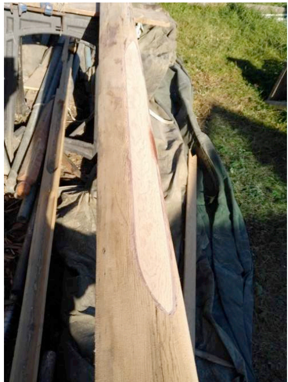
Figure 19. Spruce scarf section at spreaders.
