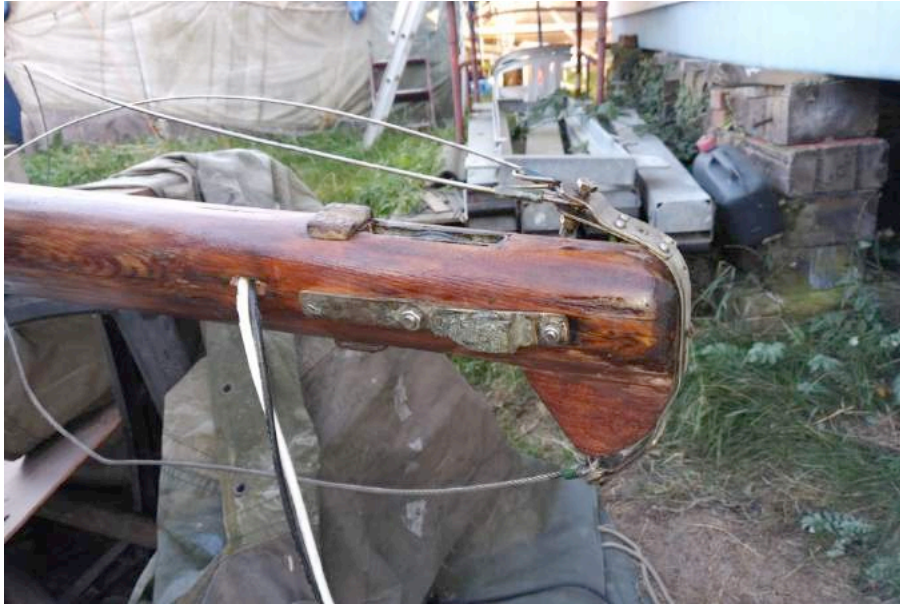
Figure 24. Cable routing mast head.
