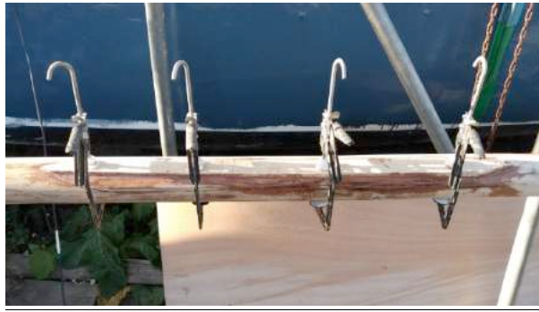
Figure 17. Spruce scarf section epoxy glued – spreaders.
