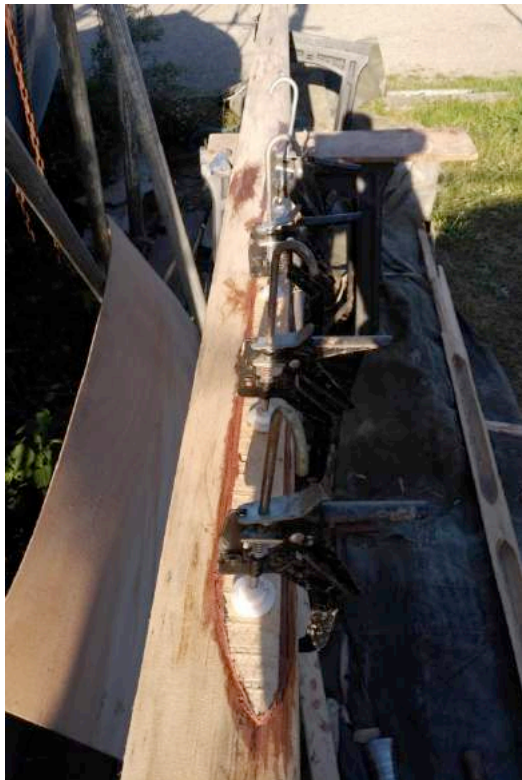
Figure 18. Another view of Spruce scarf section epoxy glued.
